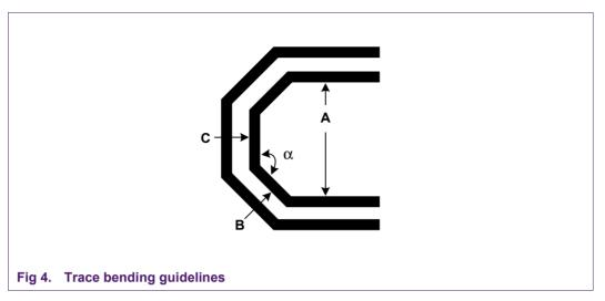
The number of left and right bends should be as close to equal as possible, to minimize the length mismatch.
