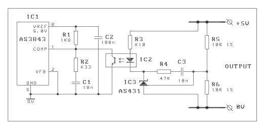
Fig 1 - Using an AS431 as an error amp.
