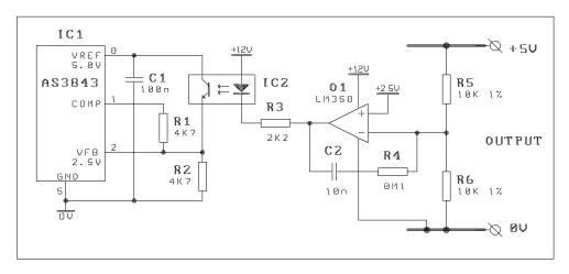
Fig 2 - Using an LM358 as an error amp.
