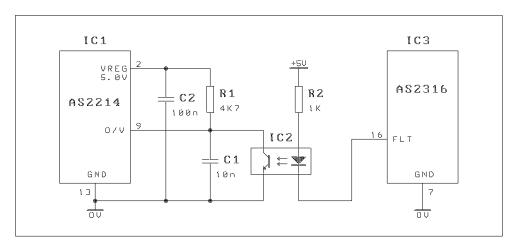
Fig 3 - A typical fault protection circuit.
