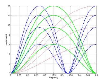
Figure 8.4.1 Frequency Response for Peaking Filters
