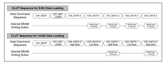
Figure 8.6.1.1 CLUT Programming Sequence Through Host Interface
