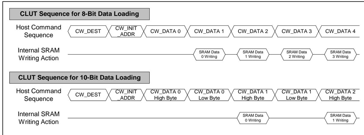
**Figure 8.6.1.1 CLUT Programming Sequence Through Host Interface**
