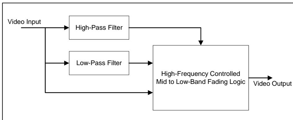
**Figure 8.3.1 VX8812 VNR Engine Block Diagram**
